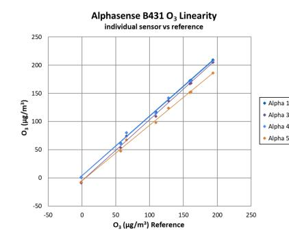
Steady-state stability SD < 2 μg/m<sup>3</sup> (calibrated)
