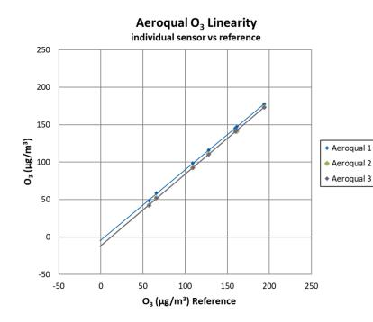
Steady-state stability SD < 2 μg/m<sup>3</sup> (calibrated)
